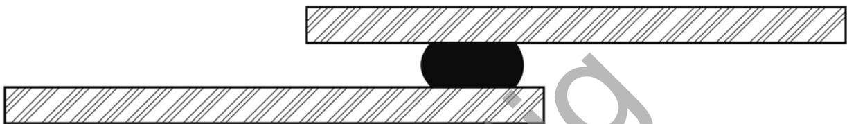
Abbildung 6: Überlappungsfuge
